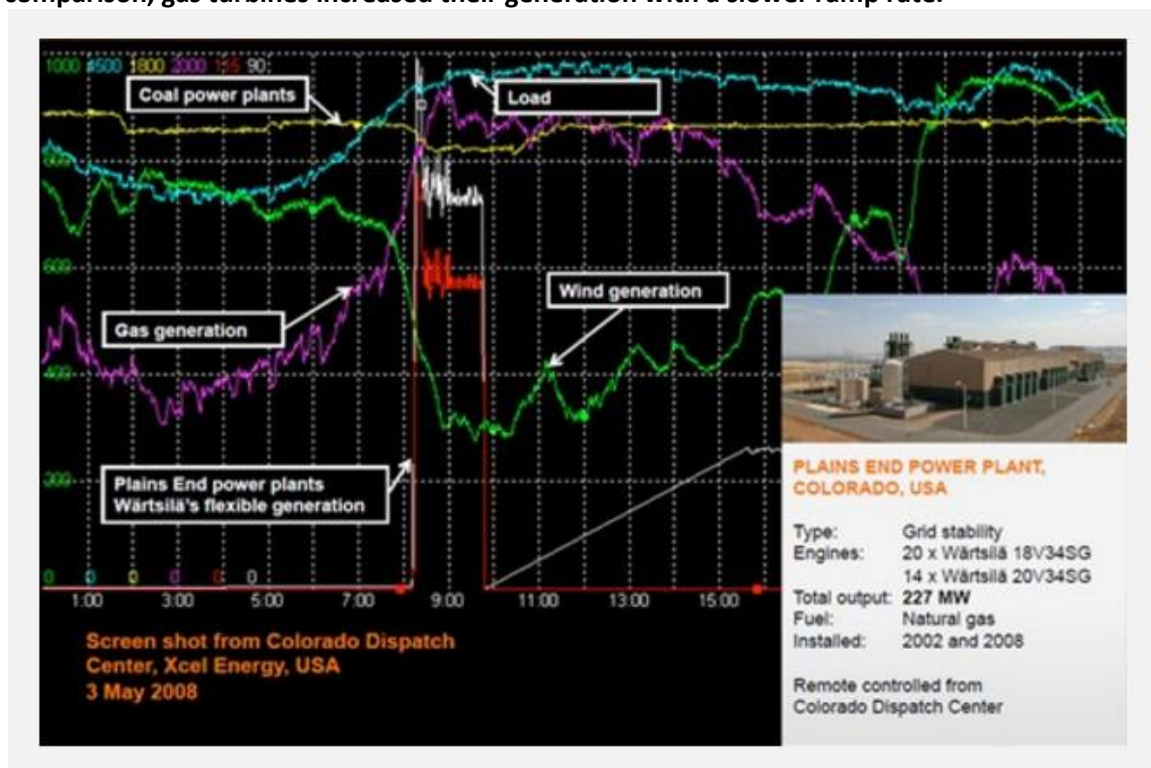
Figure 3-28: Screen shot from a dispatch center in Colorado, USA showing a drop in wind (in green) offset by a rapid rise in generation from a natural gas combustion engine power plant. In comparison, gas turbines increased their generation with a slower ramp rate.
